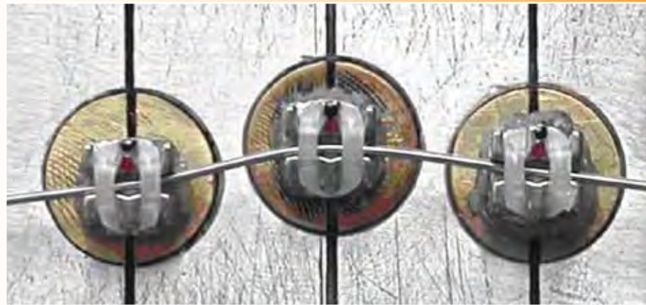
Figure 9. In-vitro model presenting the central bracket vertically (more apical) mis-aligned by 1mm compared to the other 2 adjacent brackets.
